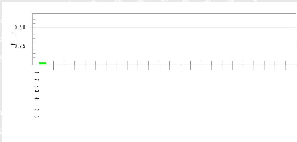
**Parameter values recorded during the test:****Vrms at the end of test (Volt): 230.01****T-max (mS): 0****Highest dc (%): 0.00****Highest dmax (%): 0.00****Highest Pst (10 min. period): 0.073****Highest Plt (2 hr. period): 0.032****Test limit (mS): 500.0****Test limit (%): 3.30****Test limit (%): 4.00****Test limit: 1.000****Test limit: 0.650****Pass****Pass****Pass****Pass****Pass**
