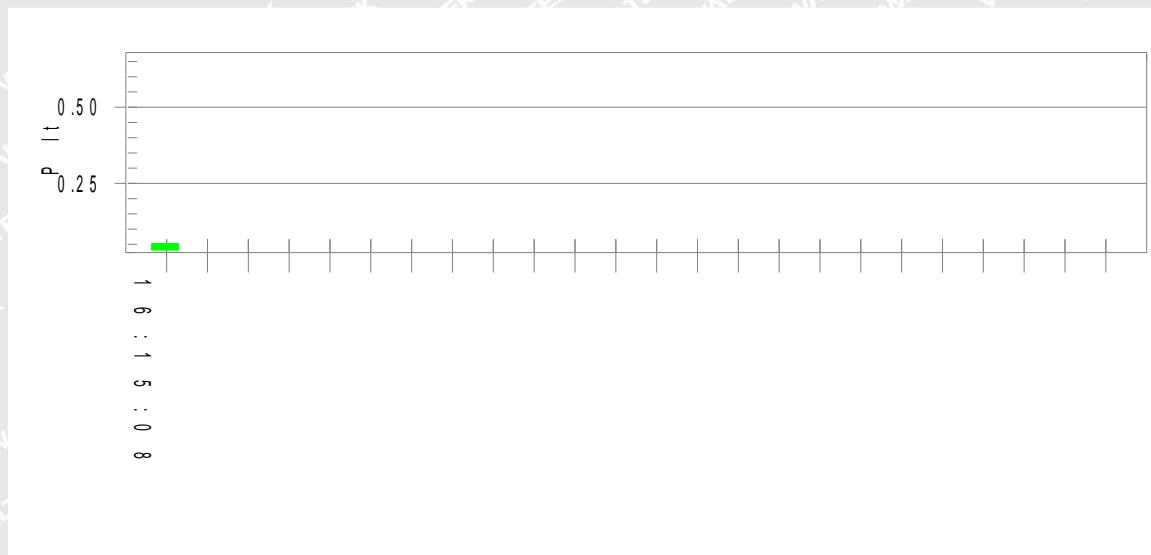
**Parameter values recorded during the test:****Vrms at the end of test (Volt): 229.66****T-max (mS): 0****Highest dc (%): 0.00****Highest dmax (%): 1.50****Highest Pst (10 min. period): 0.121****Highest Plt (2 hr. period): 0.053****Test limit (mS): 500.0****Test limit (%): 3.30****Test limit (%): 4.00****Test limit: 1.000****Test limit: 0.650**
