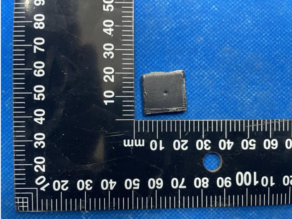
球壓試片(插頭基座: Sabc Innovative Plastics B V / CX7211(GG))
