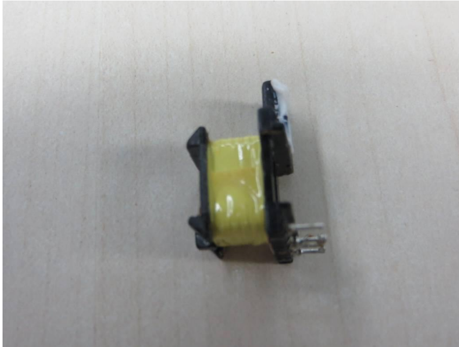
Photo 17: Internal view of transformer
