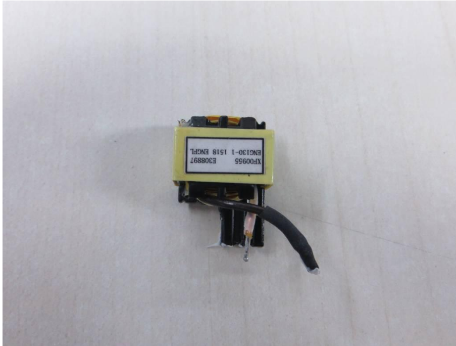
Photo 11: External view of transformer
