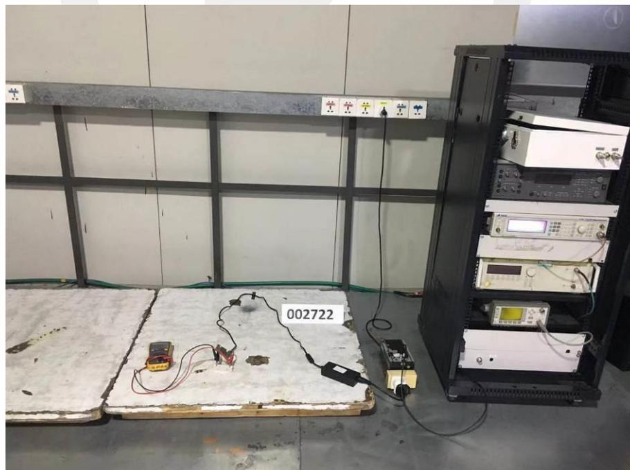
16.9.Photo of Power Frequency Magnetic Field Test
