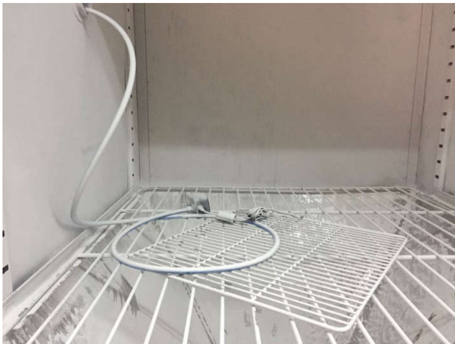
Photo 4: IP5X test for EUT
