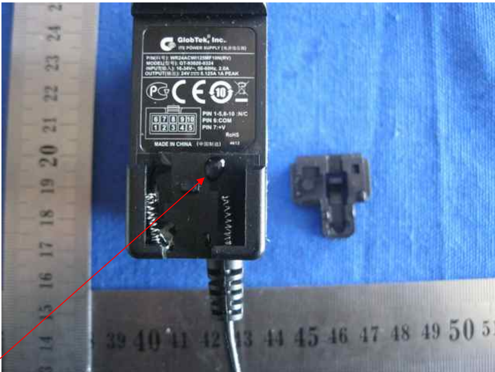
Sample after IPX1 test, Model 4 GT-93020-0324, Sample No. 2013030101-5
