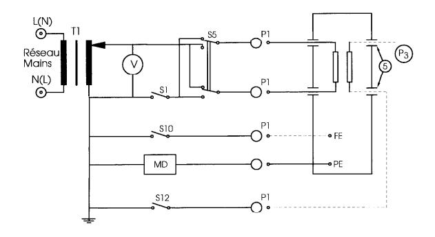
(Measuring supply circuit with one side of the supply mains at approximately earth potential (fig. 10)).
