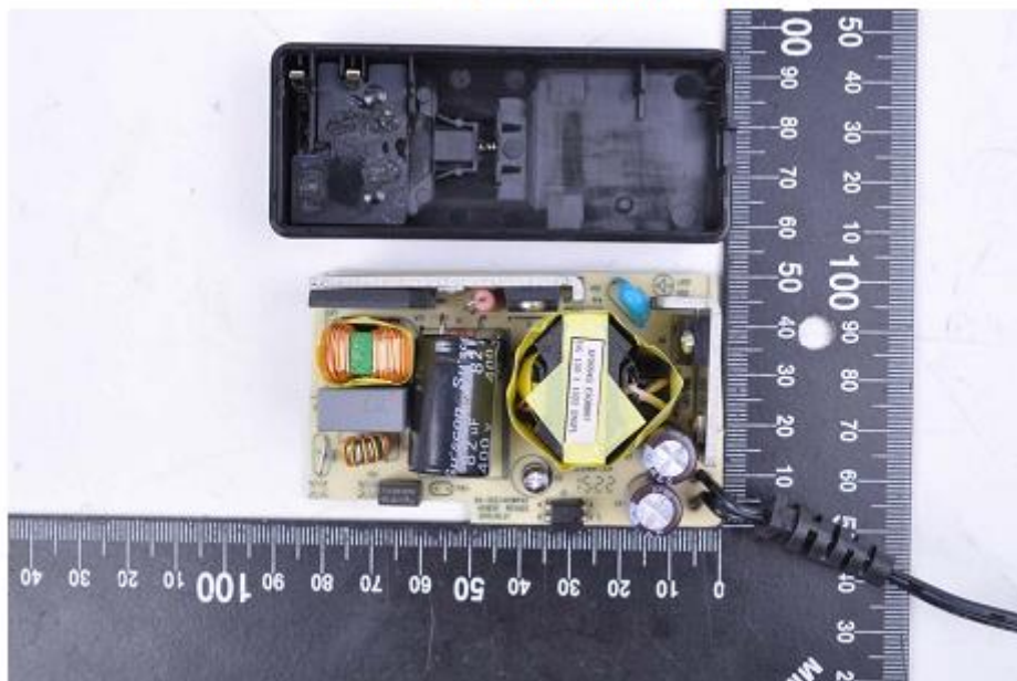
Inside view with input connection use shrapnel clip (Replaceable plug)
