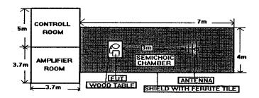
NOTE: The SPORTON 7m x 4m x 4m semichoic chamber is compliance with the sixteen points uniform field requirement as stated in IEC 1000-4-3 Section 6.2.
