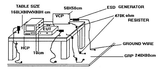
The test setup consists of the test generator, EUT and auxiliary instrumentation necessary to perform DIRECT and INDIRECT application of discharges to the EUT as applicable, in the follow manner:
