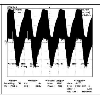
Input voltage: 240 Va.c.; 50 Hz Test Condition was : Rated output load Minus of the output, Neutral and PE were connected to simulate TN mains system.
