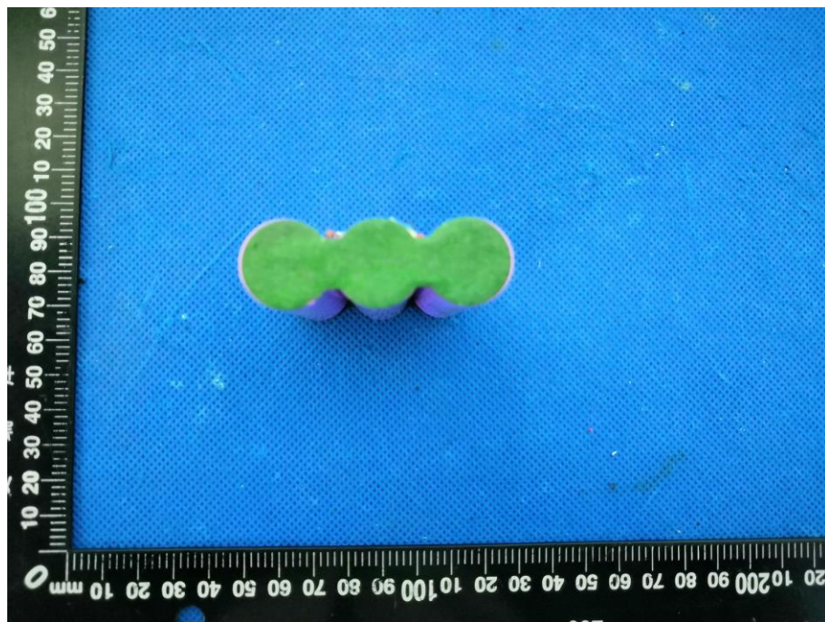
Figure 4 Internal view-2 of battery
