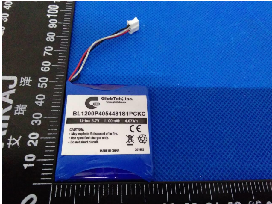
Figure 1 Front view of battery (The final version of the label, see page4 of the report)
